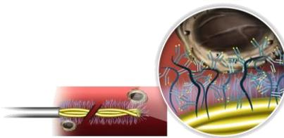
**Figure 2:** The functionalized surface of the stainless steel wire consists of a gold layer and a hydrogel incorporated with antibodies against epithelial cell surface marker EpCAM. During the application the 40 mm special coated tip comes into direct contact with the blood circulation.
